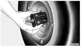
**Squeezing Winch Retainer Tabs**
