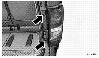
Tail Lamp Housing Fastener Removal
