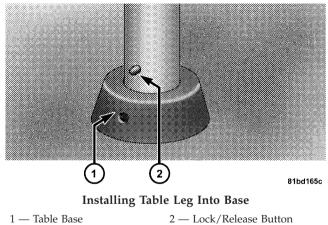
5. Twist the pole in a clockwise rotation until it stops.
