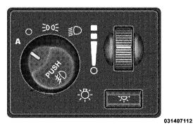
Headlight Switch With Halo Control Assembly
