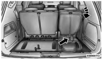
Tailgate Positioning Release Straps 2 and 32. To restore the seat to its upright position, lift up on theseatback and push forward until the anchors latch.
