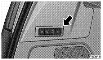
**One Touch Folding Seat Third Row** The rear switch bank allows multiple power folding and unfolding positions for the third row seats. Left and right third row seats can be folded individually or together. The third row power folding seat adjusts to the following positions using the switch bank located on the left rear trim panel:
