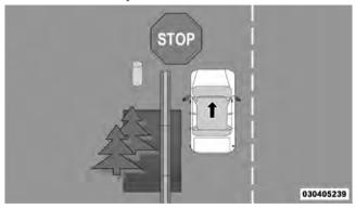
The BSM system will not alert you of objects that are traveling in the opposite direction of the vehicle in adjacent lanes.
