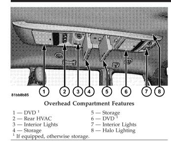
Rear Courtesy/Reading Lights — If Equipped The overhead console has two sets of courtesy lights. The lights turn on when a front door, a sliding door or the liftgate is opened. If your vehicle is equipped with Remote Keyless Entry (RKE) the lights will also turn on when the UNLOCK button on the RKE transmitter is 3 pressed.
