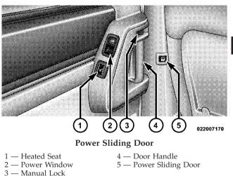
If the inside or outside door handles are used while the power sliding side door is activated, the power sliding door feature will be canceled.
