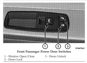
If you press the power door lock switch while the sliding door is open, the sliding door will lock.
