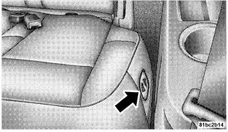
Third Row Power Seat Switch Third Row Power Seat Switch — If Equipped A one-touch power folding seat switch is located in the left rear trim panel as part of a switch bank.
