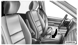
Inserting Latch Plate into Buckle
