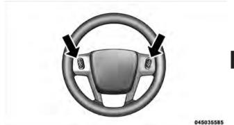
Remote Sound System Controls (Back View Of Steering Wheel)
