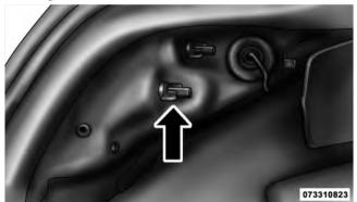
3. Grasp the tail lamp and pull firmly outward pushing on the studs from inside to disengage the lamp housing.
