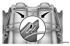
7. Align the pins at the front of the large frame with the hole in each trim panel. Slide the pins outward until fully extended into each hole.
