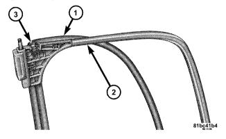
4. Pivot the small frame (1) away from the large frame (2) until the pivot lock (3) engages to lock the two frames in an L shape.
