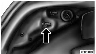
NOTE: Placing a small flat head screwdriver or similar tool between the lamp outboard ball stud and plastic grommet from inside the trunk can help to disengage the outboard edge of the tail lamp.
