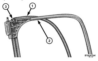
4. Pivot the small frame (1) away from the large frame (2) until the pivot lock (3) engages to lock the two frames in an L shape.
