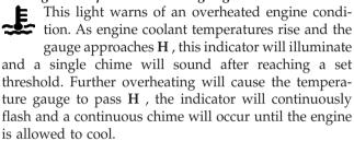
If the light turns on while driving, safely pull over and stop the vehicle. If the A/C system is on, turn it off. Also, shift the transmission into NEUTRAL and idle the vehicle. If the temperature reading does not return to normal, turn the engine off immediately and call for service. Refer to "If Your Engine Overheats" in "What To Do In Emergencies" for further information.
