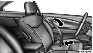
**Inserting Latch Plate Into Buckle**
