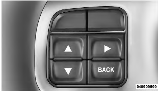
EVIC Steering Wheel Buttons
