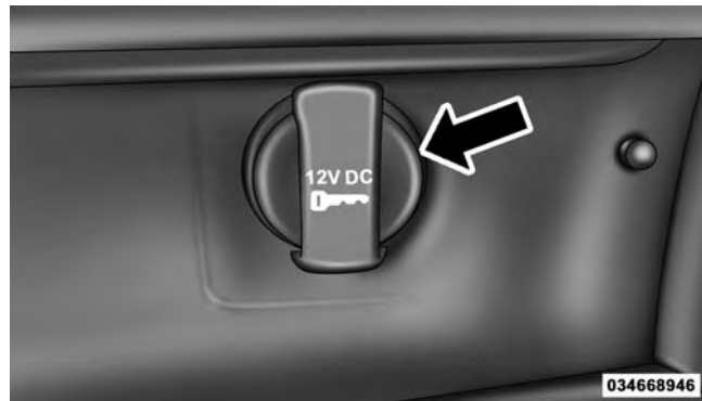
Front Power Outlet
