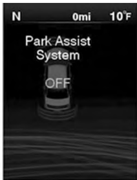
Park Assist System OFF
