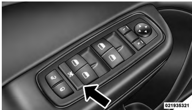
Window Lockout Switch
