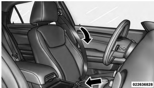
Pulling Out The Lap/Shoulder Belt Latch Plate
