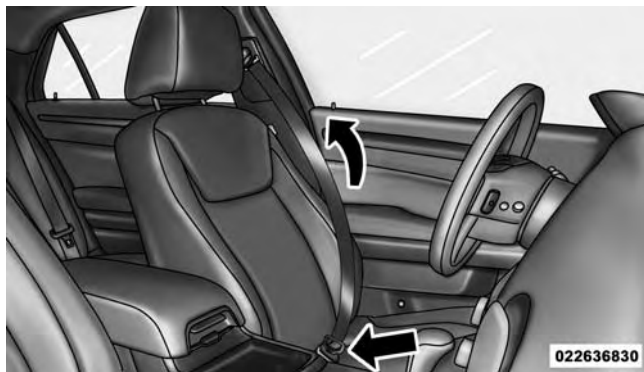
Removing Slack From Belt
