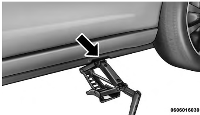
Jack Engaged (Rear Jacking Location)
