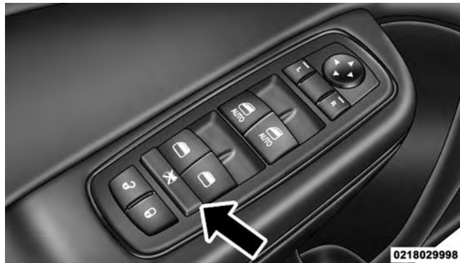
Window Lockout Switch
