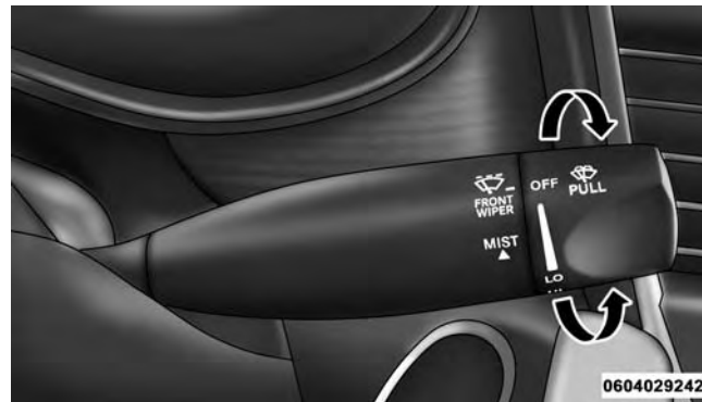
Windshield Wiper Operation
