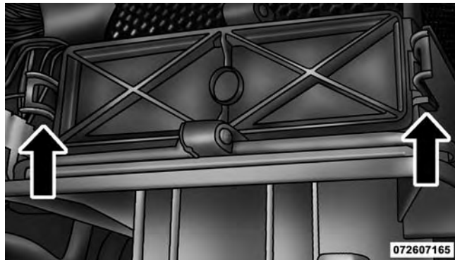
A/C Air Filter Replacement
