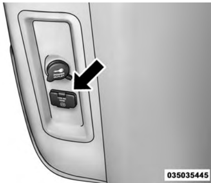
Power Inverter Outlet
