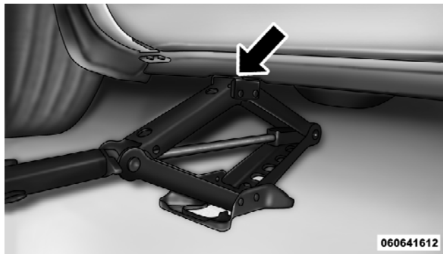
Front Jacking Location
